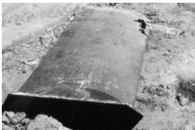
Fig. 2 C100 blade erosion after four years
